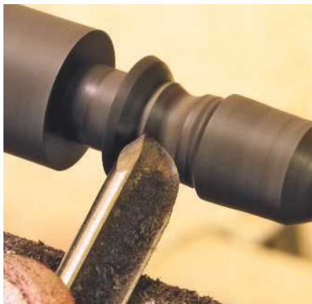
▲ Pic.26 The gouge is an easier tool to use on the spindle than the skew chisel. You can even do the fillets with the tool. Here the gouge is rolled round to do the small cove at the base of the finial
